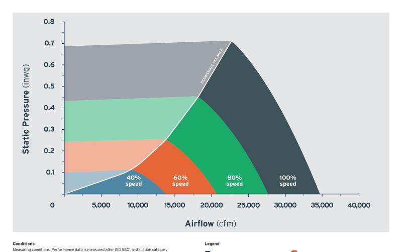
Measuring conditions: Performance data is measured after ISO S8UI, installation category A, as a complete axial fan without fan guard. Data refer to air density 0.075lb/ft3 (68° sea level). Sound data is measured at suction-side. The data apply only under the specified measuring conditions and may change due to installation conditions. In case of deviations from the standard design, the characteristic values must be checked in the installed
