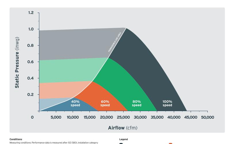
A, as a complete axial fan without fan guard. Data refer to air density 0.075lb/ft<sup>3</sup> (68° sea level). Sound data is measured at suction-side. The data apply only under the specified measuring conditions and may change due to installation conditions. In case of deviations
